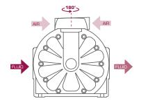
Orientable air inlet, increased installation flexibility.
