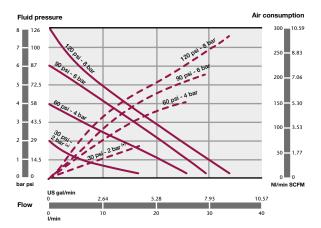
(\*) 30 psi test with a PTFE (Teflon®) diaphragms pump.
