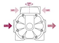
Orientable air inlet, increased installation flexibility.
