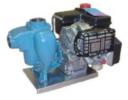
The unique FLOMAX PUMPAK design permits close coupling to a wide range of gas and diesel engines. FLOMAX pumps include a stainless steel shaft sleeve to protect the engine crankshaft from damage. The open adaptor allows for the proper ventilation and operating temperature of the engine bearing while providing separation between the engine and the liquid in the pump.
