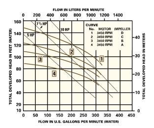
To use the chart, locate your required operating point (intersection GPM & TDH). If the operating point is between two curves, select the higher of the two. The required motor horsepower will be shown by the first diagonal line to the right of the operating point.
