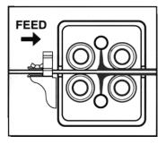
Independent manifold valves permit application of lubricant to either top, bottom or both sides simultaneously. There is no waste with a Graymills Stocklube System because unused lubricant is recirculated.
