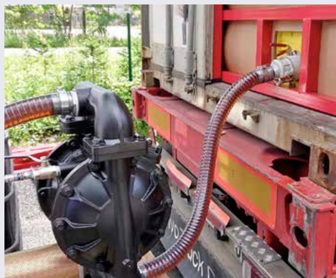
High fluid viscosity reduces pump delivery.
